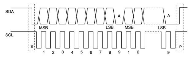
S; Start condition, a high to low transition of the SDA line while SCL is high P: Stop condition, a low to high transition of the SDA line while SCL is high
