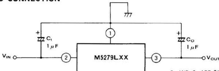
C<sub>1</sub> AND C<sub>2</sub> ARE CAPACITORS TO PREVENT OSCILLATIONS.
