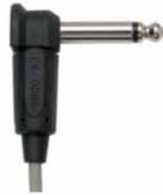
Phone jack: In each series the probe (thermistor) is connected to a 10 ft (3 M) long cable with a two-conductor, 0.250 in (6.35 mm) diameter phone style plug. It is also available in a straight-molded phone plug.
