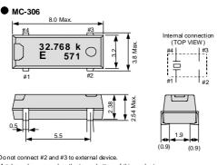
Do not connect #2 and #3 to external device. Metal may be exposed on the top or bottom of this product. This will not affect any quality, reliability or electrical spec.
