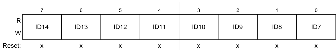
Figure 12-25. Identifier Register 2 (IDR2) — Extended Identifier Mapping
