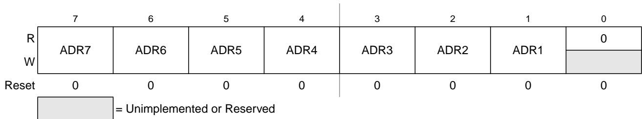
Figure 11-2. IIC Bus Address Register (IBAD)
