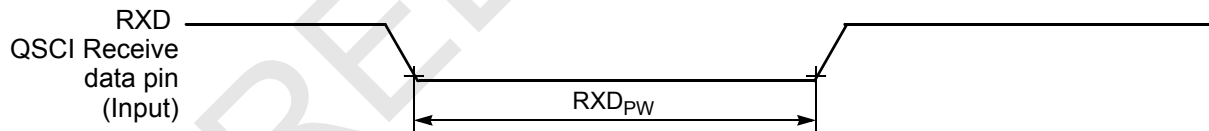
Figure 10-12 RXD Pulse Width
