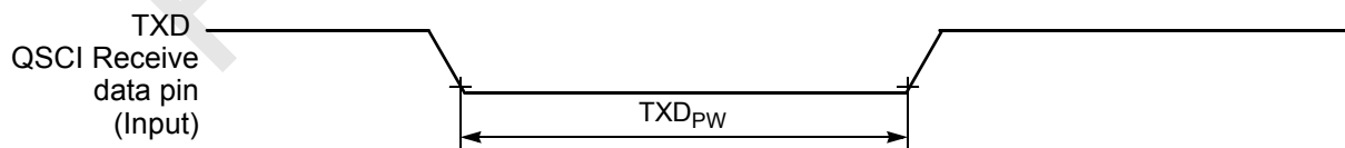
Figure 10-13 TXD Pulse Width
