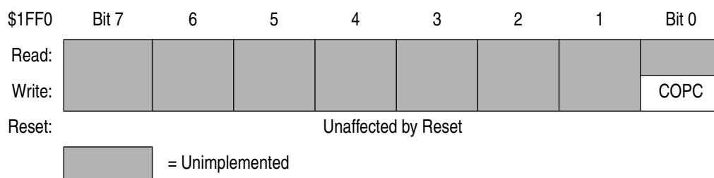
Figure 10-4. COP and Security Register (COPR)
