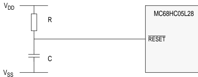
Figure 2-4 RC connection for external POR
