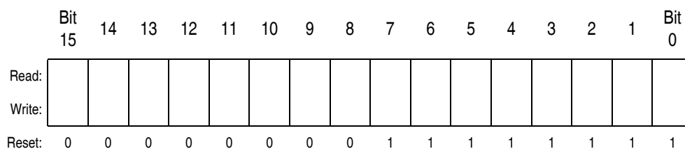
Figure 7-4. Stack Pointer (SP)
