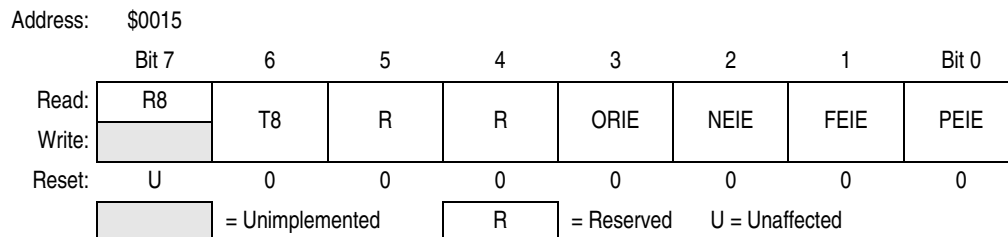
Figure 13-12. ESCI Control Register 3 (SCC3)
