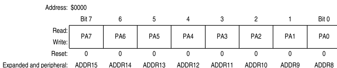
Figure 6-1. Port A Data Register (PORTA)
