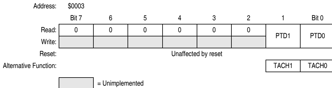
Figure 12-10. Port D Data Register (PTD)
