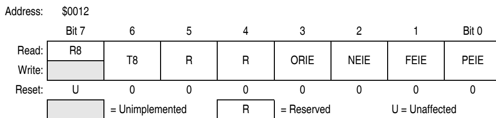
Figure 13-11. ESCI Control Register 3 (SCC3)
