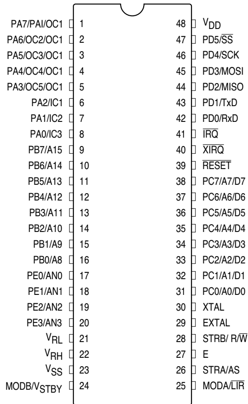
Figure 3 48-Pin DIP Pin Assignments
