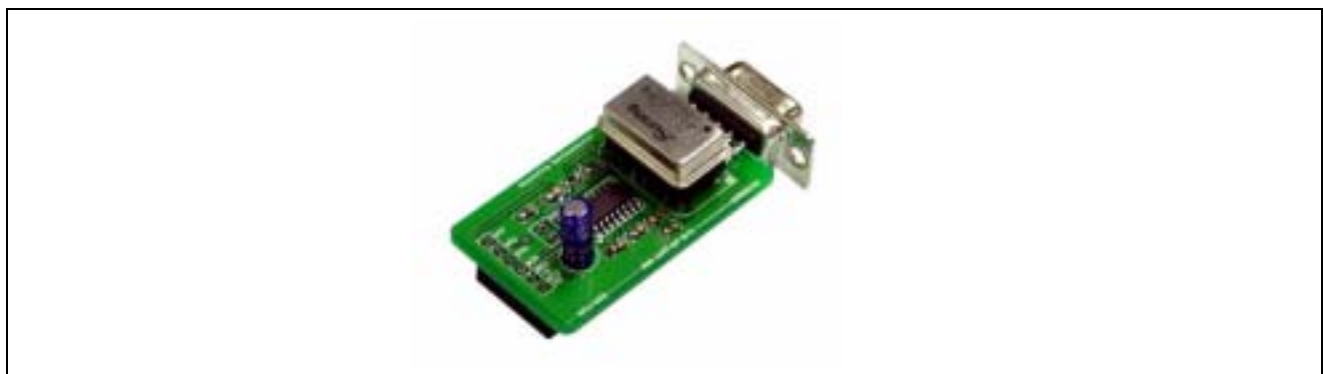
Figure 27-3 MagnaChip supplied ISP Board
