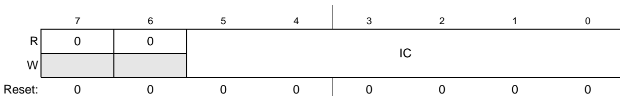
Figure 24-3. I 2 C Frequency Divider Register (I2FDR)
