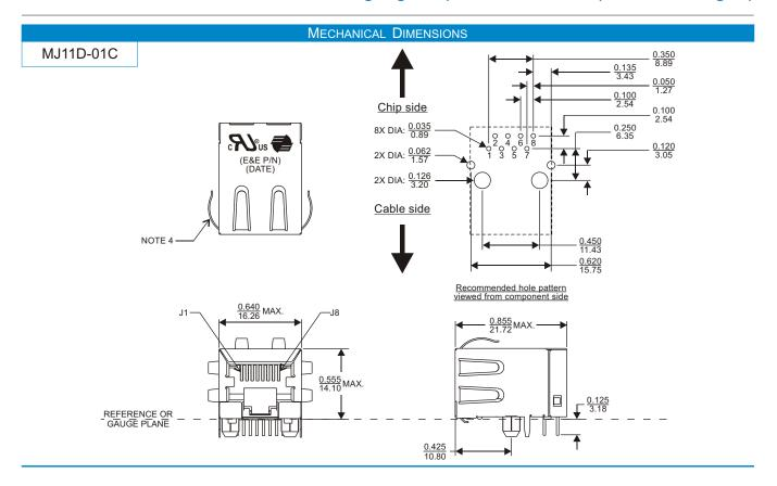
All dimensions are specified in  $\frac{\text{inch}}{\text{mm}}$  with higher precedence in inch. Unless otherwise specified, all tolerances are  $\pm \frac{0.010}{0.25}$
