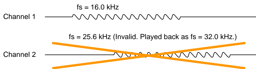
Figure 1 In Case a Different Sampling Frequency Played Back during Playback of the Other Channel Playback
