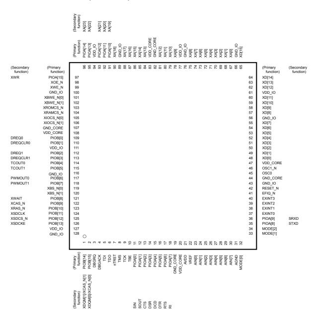
128-Pin Plastic TQFP
