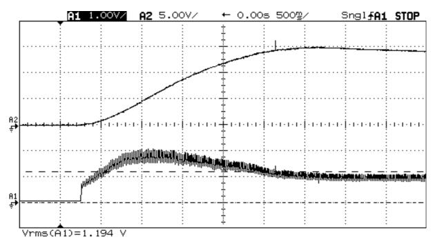
In the second plot we directly connect the same motor to the line voltage:
