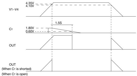
Note: When pin Ct is shorted or left open, the output goes low when overcharging is detected.
