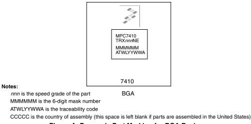
Figure A. Freescale Part Marking for BGA Device
