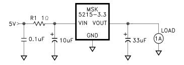
For a given continuous maximum load of 1 amp, R1 can be selected to drop the voltage seen at the regulator to 4V. This allows for the output tolerance and dropout specifications. Input voltage variations (5V) also should be included in the calculations. The resistor should be sized according to the power levels required for the application.
