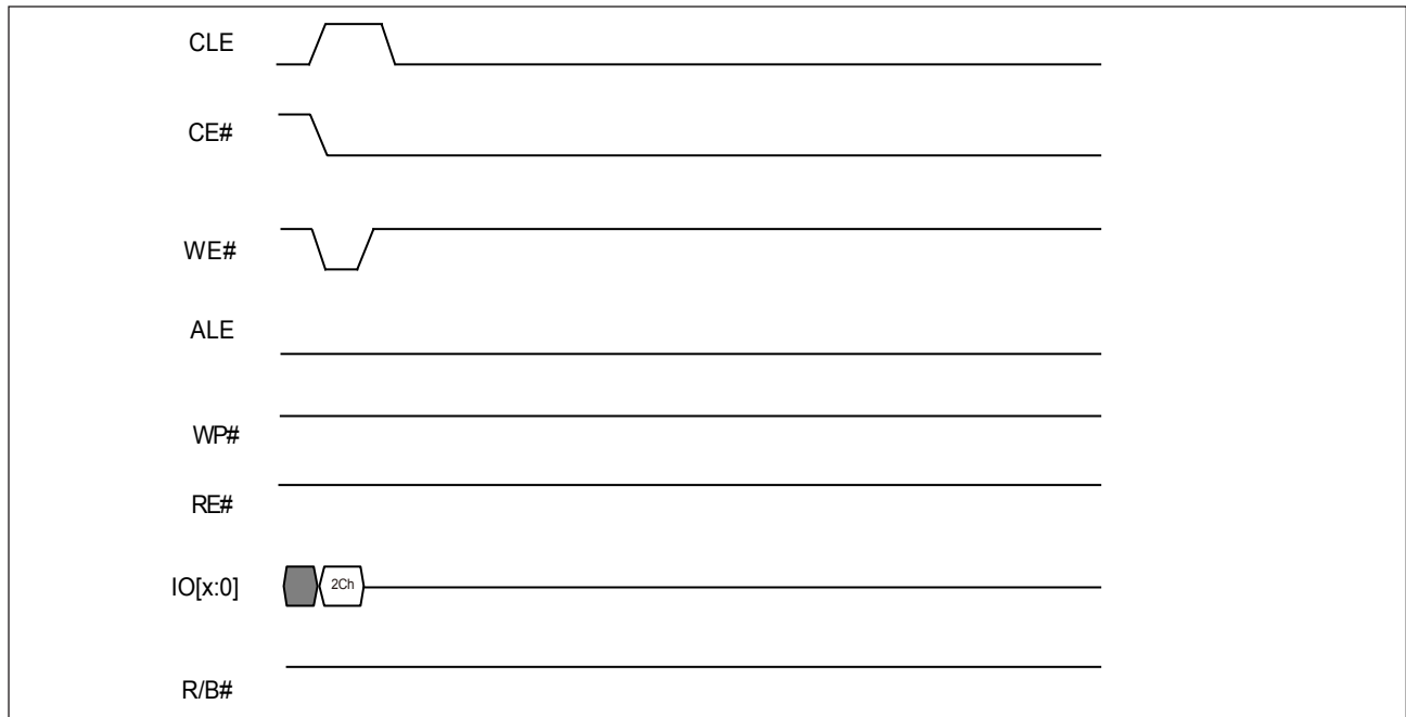
Figure 39. AC Waveforms for Block Solid-Protect
