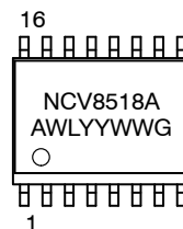
SOIC-16 LEAD WIDE BODY EXPOSED PAD CASE 751AG
