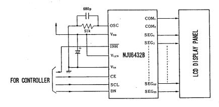
(Note) After rising edge of V<sub>DD</sub> voltage, the display data is not guaranteed and which blinking is meaningless display. Therefore, keep TNH terminal to Low Level by the display data transferred is needed.
