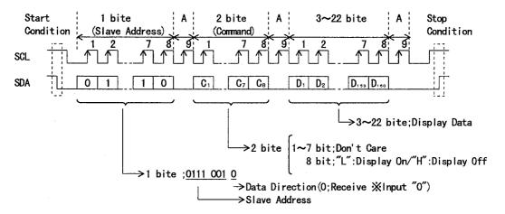
Whole 160bits data transfer to the shift register. When the input data in less than 160 bits, parts which bit data is inputed corresponded to display, and segment which correspond to the rest part in "off".
