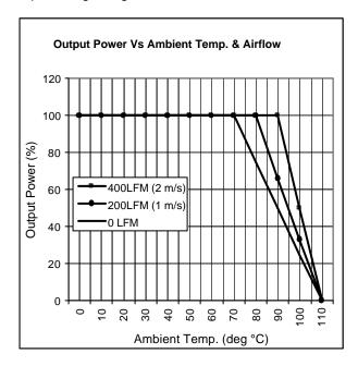
The 9-36V and 18-75V input voltage versions of this series feature a 4:1 input voltage range and can achieve operation at full power at 85°C ambient temperature with only convection cooling.
