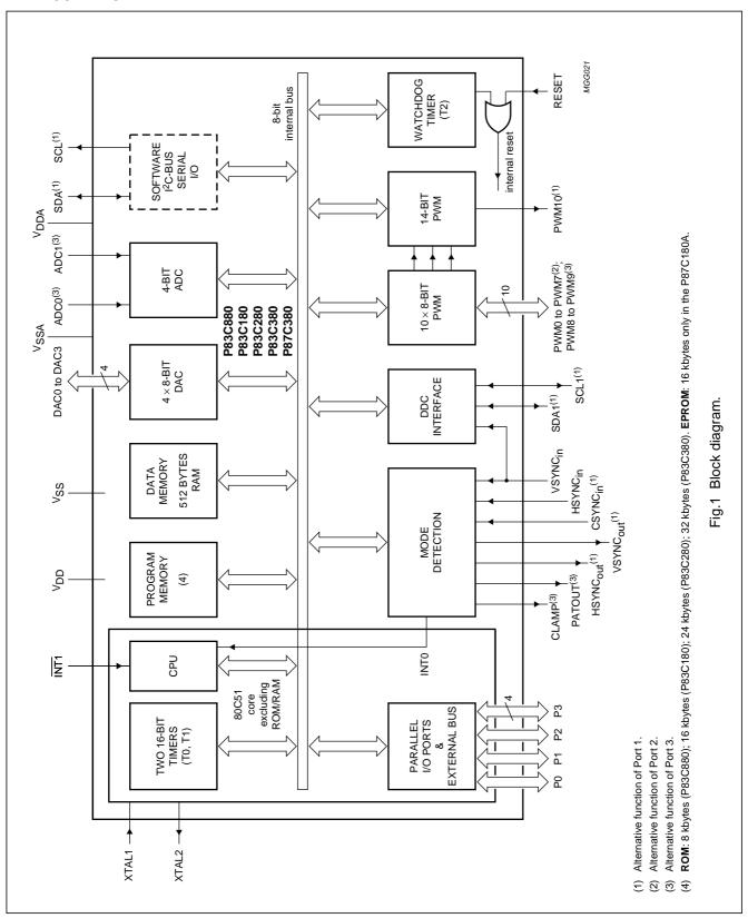
Microcontrollers for monitors with DDC interface, auto-sync detection and sync proc.
