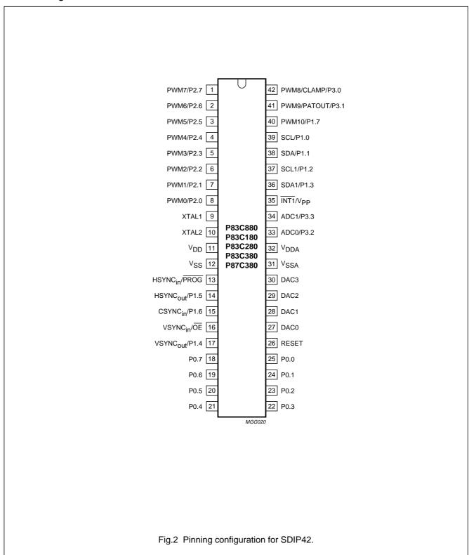
Microcontrollers for monitors with DDC interface, auto-sync detection and sync proc.
