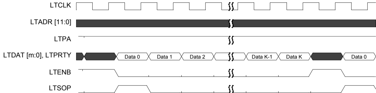
Figure 48 - Loop UTOPIA L1 Transmit Master
