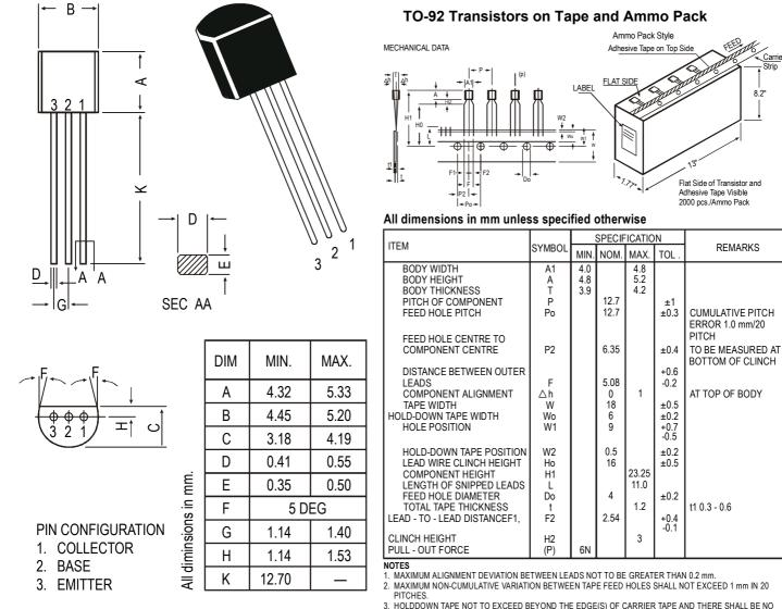
HOLDDOWN TAPE NOT TO EXCEED BEYOND THE EDGE(S) OF CARRIER TAPE AND THERE SHALL BE NO
