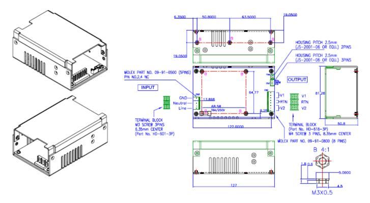
PSRL0603DF Series (Enclosed with Top Built-in Fan Type): 5(L) x 3.2(W) x 2(H) inches; Weight: 550g.
