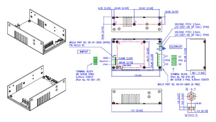
PSRL0603DU Series (U-Chassis with Type A Cover): 5(L) x 3.2(W) x 1.56(H) inches; Weight: 470g.
