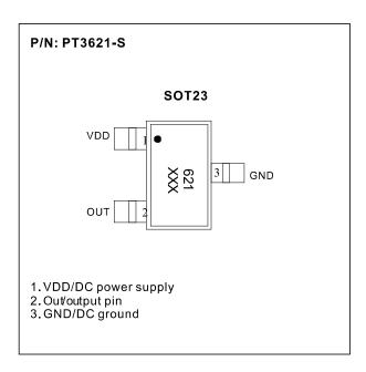
The PT3621 is designed for magnetic actuating using a unipolar magnetic field. The built-in dynamic offset cancellation of pre-amplifier stage achieves optimal symmetrical magnetic sensing. This Hall effect IC is designed for on/off detection, especially for automotive/industrial application. PT3621 provides precious actuation to ensure safety. The supply voltage range is from 2.5V to 18V and maximum output current is 25mA.
