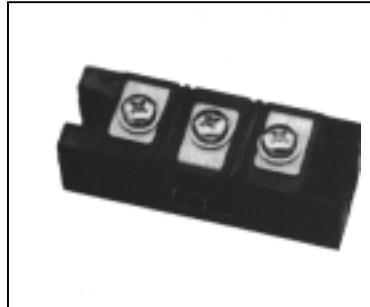
QIC0620003 Dual IGBT Module Common Emitter 200 Amperes / 600 Volts
