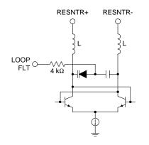
To tune the VCO the designer only needs to calculate the value of the inductors connected to pins 18 and 20 (RESNTR- and RESNTR+). The inductor value is determined by the following equation.
