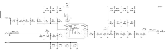
This eval board for low power linear operation:  $21 \text{dBm} < P_{OUT} < 27 \text{dBm}$ ,  $5 \text{V} \le V_{CC} \le 8 \text{V}$ . Bias R seen above for 8V and 60 mA I<sub>REF</sub>. See biasing table for setting resistance at other supply voltages.
