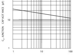
V<sub>R</sub>, REVERSE VOL TAGE (V) Fig. 4 Typical Junction Capacitance
