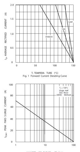
NUMBER OF CYCLES AT 60 Hz Fig. 3 Max Non-Repetitive Peak Fwd Surge Current
