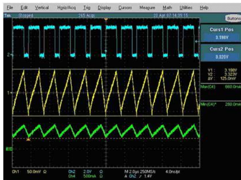
Figure 21. Electrolytic 100 \mu F (Ripple Too High)
