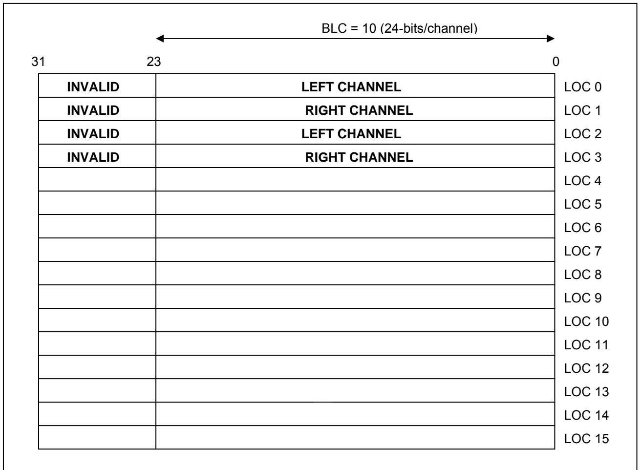
Figure 36-5. TX FIFO Structure for BLC = 10 (24-bits/channel)
