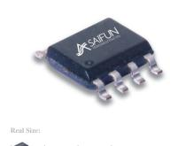
Saifun's SA25F family of SPI devices provides small-sized, cost-effective, low-power and high-performance Serial Flash memory chips for today's market needs. Using the patented Saifun NROM™ technology, the SA25F devices contain two bits per cell, which ensures minimal die size and maximal growth within the same package with increasing densities.
