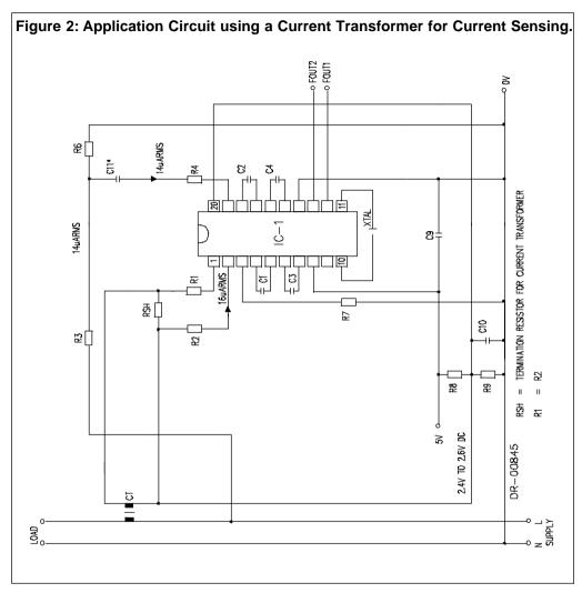
Note: Capacitor C11 may be selected for phase compensation and DC blocking.
