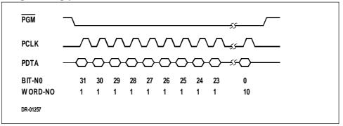
The PGM pin is pulled low and the PCLK pin should be clocked with an external clock. The programming data on the PDTA pin must be stable during the rising edge of the clock signal on PCLK.
