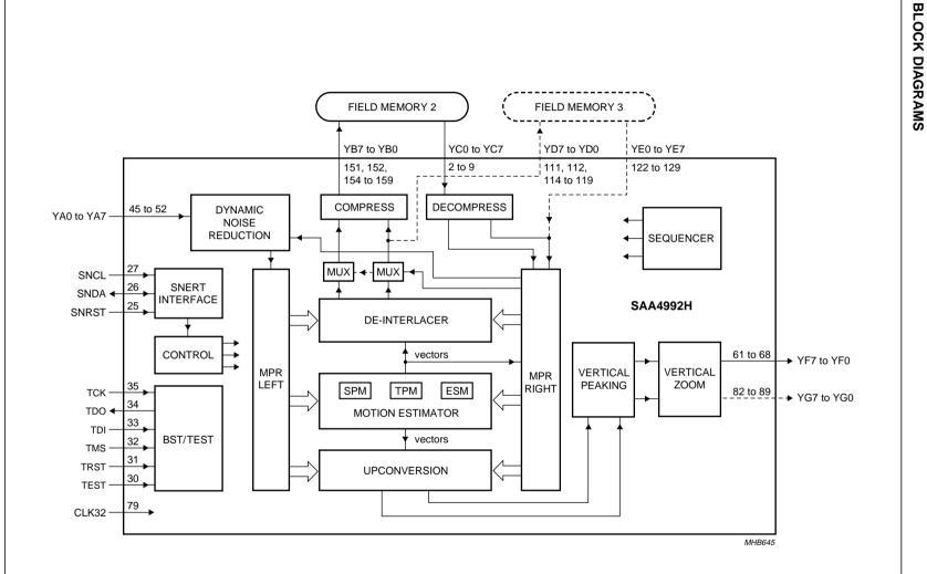
The solid lines represent pixel data; the broken lines represent controls.
