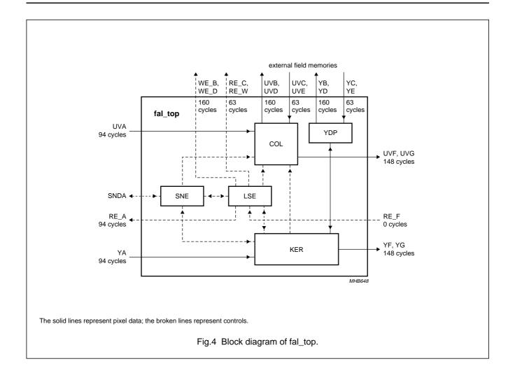
Field and line rate converter with noise reduction
