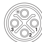
Pin assignment of M12 socket, 4-pos., S-coded, socket side view
