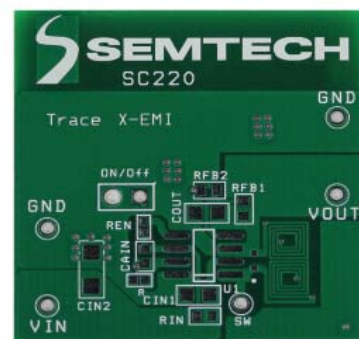
Figure 1. Top view of an evaluation board with X-EMI inductor
