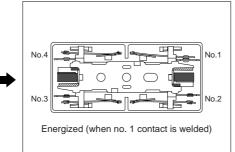
If the No. 1 contact welds. A gap of greater than 0.5 mm .020 inch is maintained at each of the two form "a" contacts (Nos. 2 and 4).
