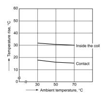
3. Ambient temperature characteristics Tested sample: SF4-DC12V Quantity: n = 6
