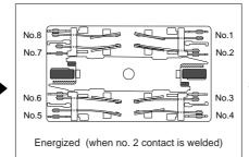
If the No. 2 contact welds. Each of the four form "a" contacts (Nos. 1, 3, 5, and 7) maintains a gap of greater than 0.5 mm
