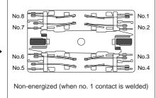
If the No. 1 contact welds. The adjacent No. 2 contact maintains a gap of greater than 0.5 mm .020 inch. The other contacts, because the coil is not energized, return to their normal return state; each of form "a" contacts (nos. 3, 5, and 7) maintains a contact gap of greater than 0.5 mm .020 inch; each of the form "b" contacts (nos. 4, 6, and 8) return to a closed
