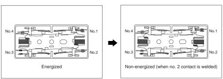
If the No. 2 contact welds. The single form "b" contact (No. 3) maintains a gap of greater than 0.5 mm .020 inch.
