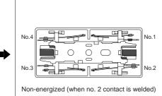
If the No. 2 contact welds. Each of the two form "b" contacts (Nos. 1 and 3) maintains a gap of greater than 0.5 mm .020 inch.
