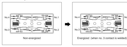
If the No. 3 contact welds. Each of the two form "a" contacts (Nos. 1, 2, and 4) maintain a gap of greater than 0.5 mm .020 inch.
