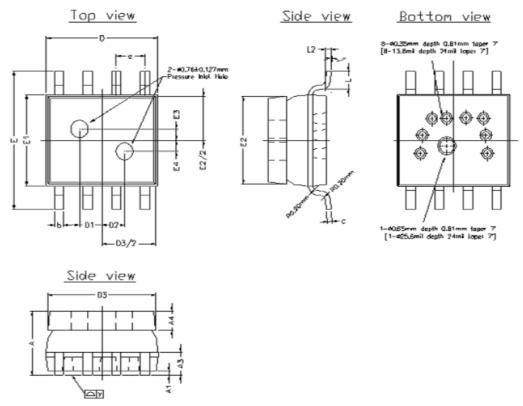
Note: Contact factory for specific location and type of pin 1 identification.
