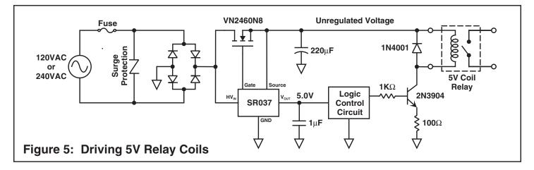
The circuit shown in Figure 5 uses the SR037 to supply a regulated 5.0V for the logic control circuitry while the unregulated voltage is used to drive a 5.0V coil relay. To overcome the voltage variation of the unregulated line, a bipolar transistor is
