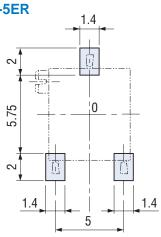
Note) The zero point is the center of mounting.
