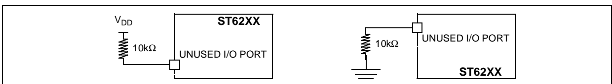
Figure 56. Two typical Applications with unused I/O Pin
