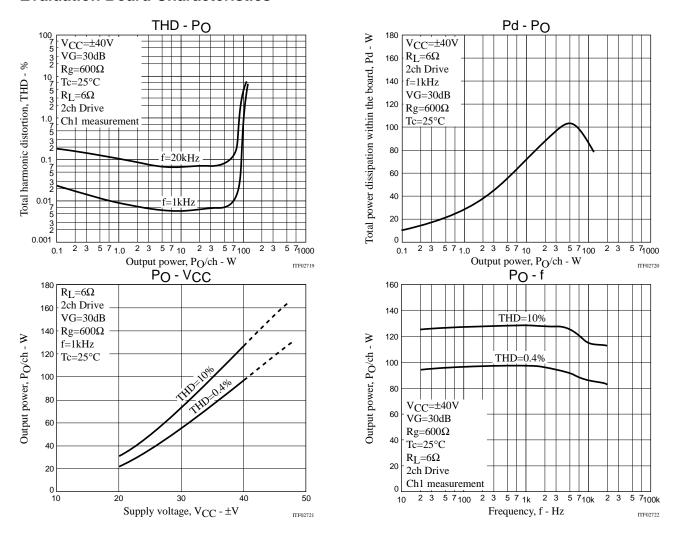
[Thermal Design Example for STK433-120-E (R<sub>L</sub> =  $6\Omega$ )]
